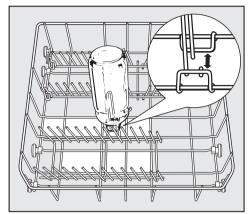
The bottle holder, e.g. for milk and baby bottles, can be inserted in various positions in the lower basket. See areas marked white in the illustration. However, do not place a bottle holder in the middle or in the corners. Water will not be able to access the bottles properly, and cleaning results will be impaired.
